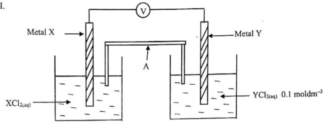
The above figure defict a cell constructed using metal X and Y dipping in their own metal ion solution.
